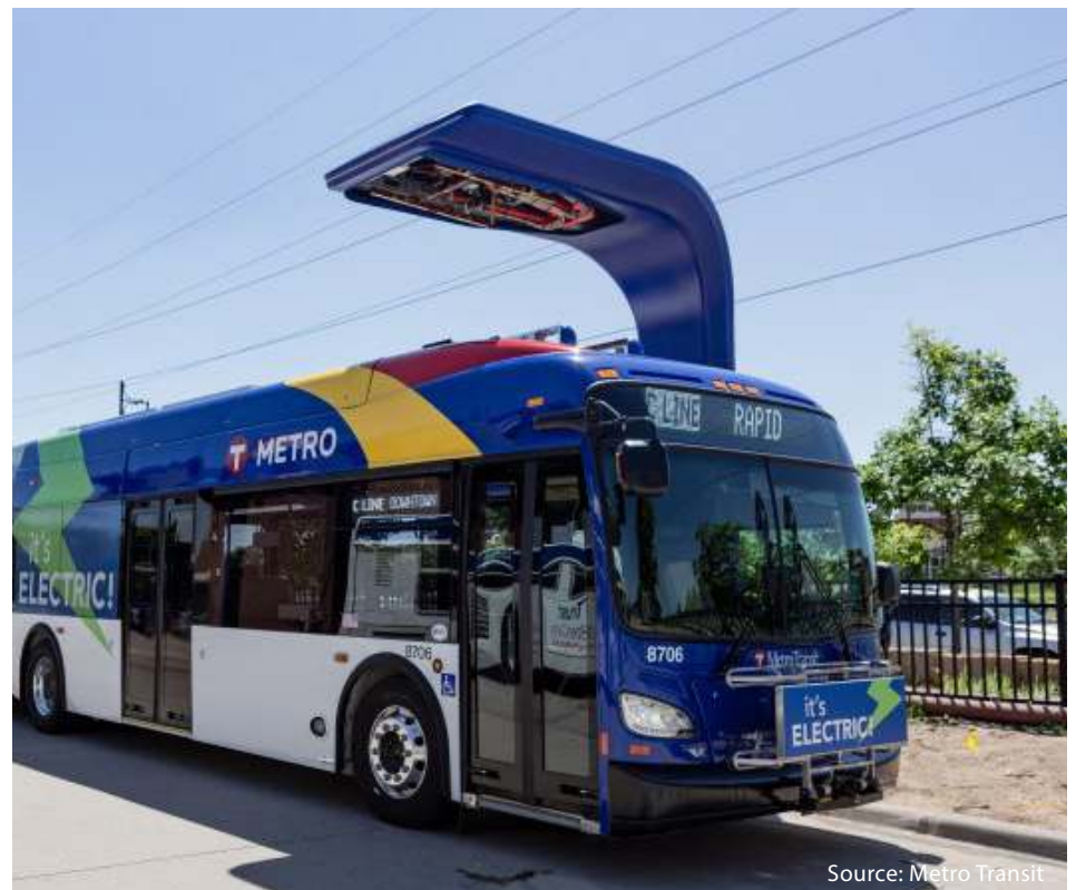
Figure 103: Transit electric charging station – C Line
