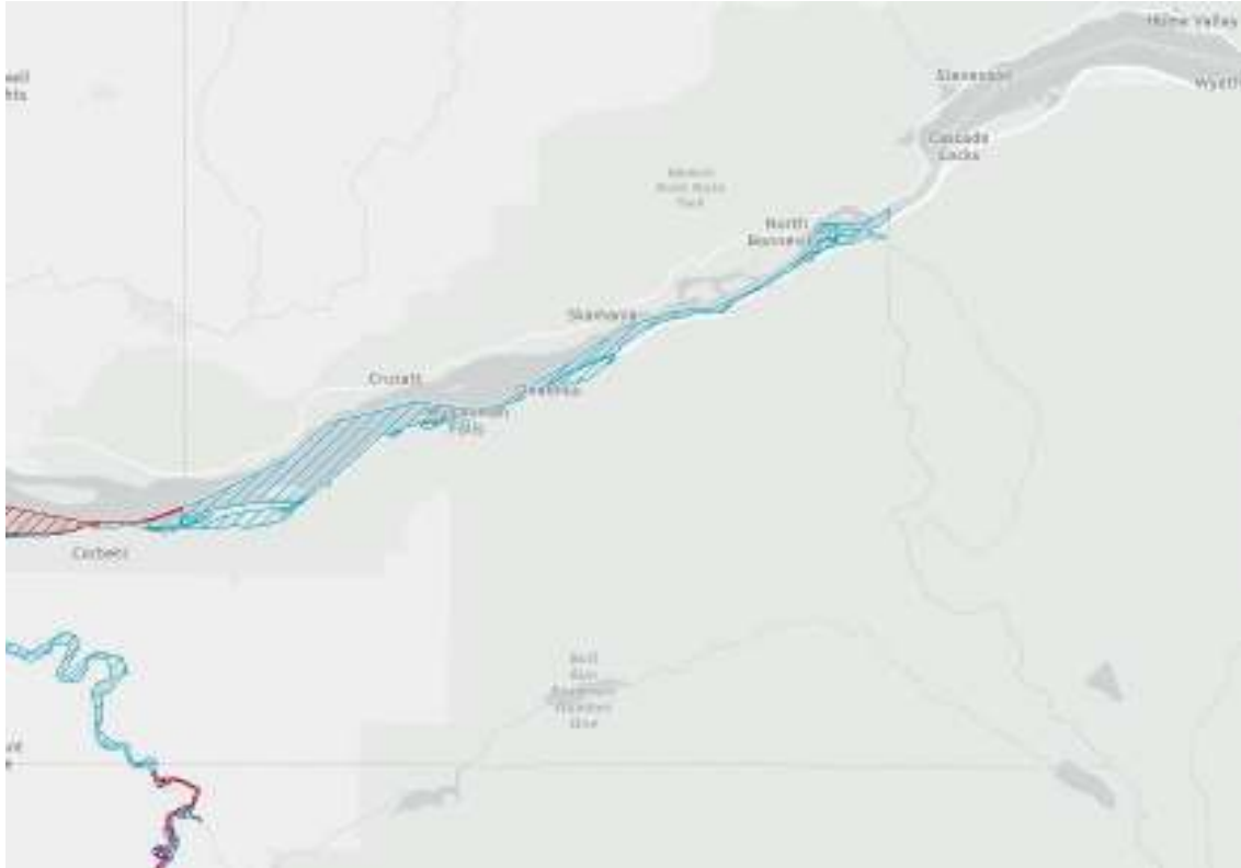
Figure 49 – DOGAMI Map showing FEMA identified flood risk zones in the eastern portion of Multnomah County. The areas hatched in red are floodways, the blue hatched areas are the Special Flood Hazard Area, and the purple areas are the 0.2% annual chance flood areas where regulation is optional. FEMA's National Flood Hazard Layer is the most up to date source for property-specific flood hazard designations.
