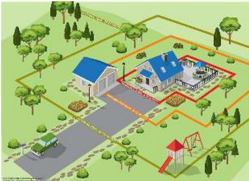
Figure 104 - A diagram of the home ignition zone, where work can be done to make it less likely a structure will ignite in a wildfire. Each zone has specific recommendations. Graphic from the National Fire Protection Association
