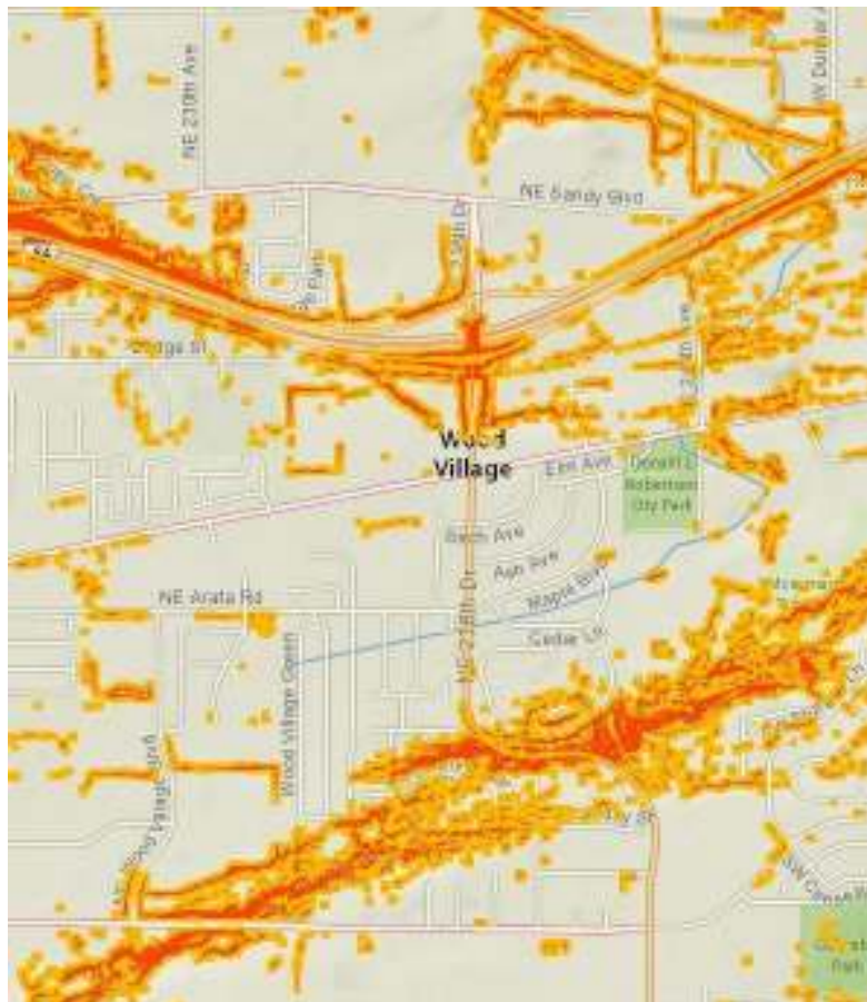
Figure 152 - Map showing shallow landslide risk in the City of Wood Village. The darker color of orange represents areas with higher risk. Map - DOGAMI SLIDO map.
