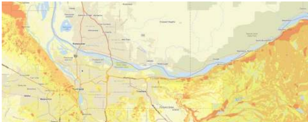
Figure 177 - Map showing landslide risk across Multnomah County. Red has the highest risk, orange is moderate risk and yellow areas have lower risk. Map from DOGAMI SLIDO site.
