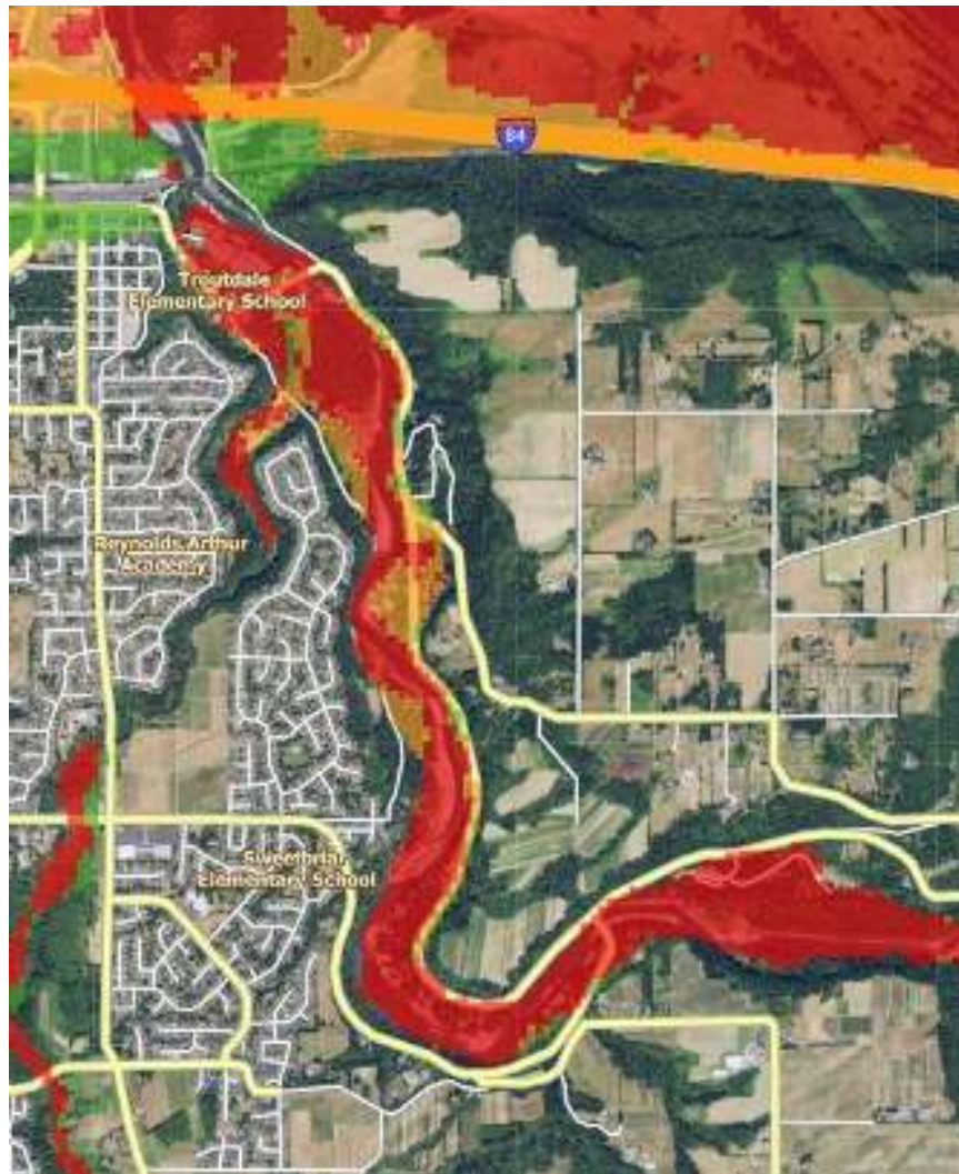
Figure 168 - Map showing soil liquefaction risks around Sandy River bridges. Red indicates high soil liquefaction risk, orange is moderate risk, and green are lower risk. Map from DOGAMI HazVu site.
