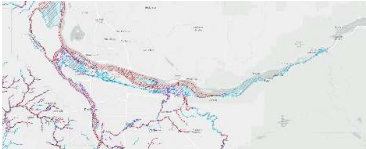
Figure 11 - Map showing areas mapped by FEMA's National Flood Insurance Program (NFIP). Areas in red hatching are the regulatory floodway, areas with the fastest and most dangerous floodwaters during a flood. The blue areas are those predicted to flood in a 1% annual chance (100 year) flood. Purple areas are those predicted to flood in a 0.2% annual chance (500 year) flood. Map from DOGAM's HazVu website, with information from FEMA's National Flood Hazard Layer (NFHL) .
