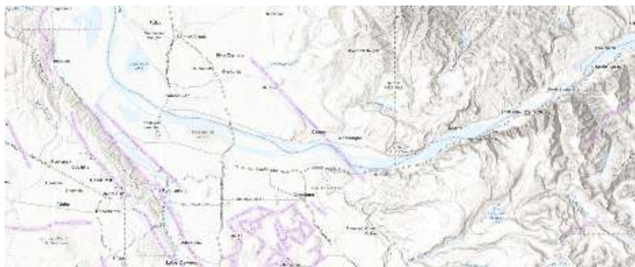
Figure 28 - Map showing known earthquake faults in Multnomah County. Map hosted on DOGAMI's HazVu website.
