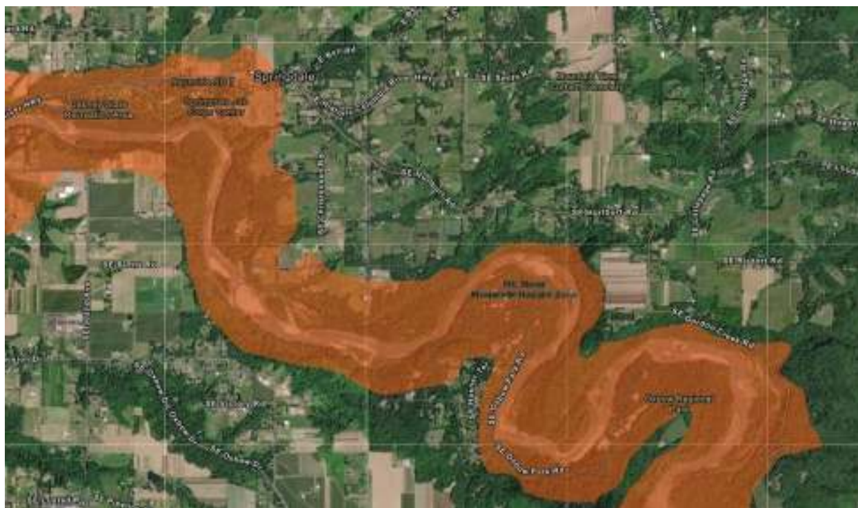
Figure 179 - Map showing potential lahar impacts from an extra-large eruption of Mount Hood. The orange areas would be inundated by debris in this volcano scenario. Map from DOGAMI HazVu site.
