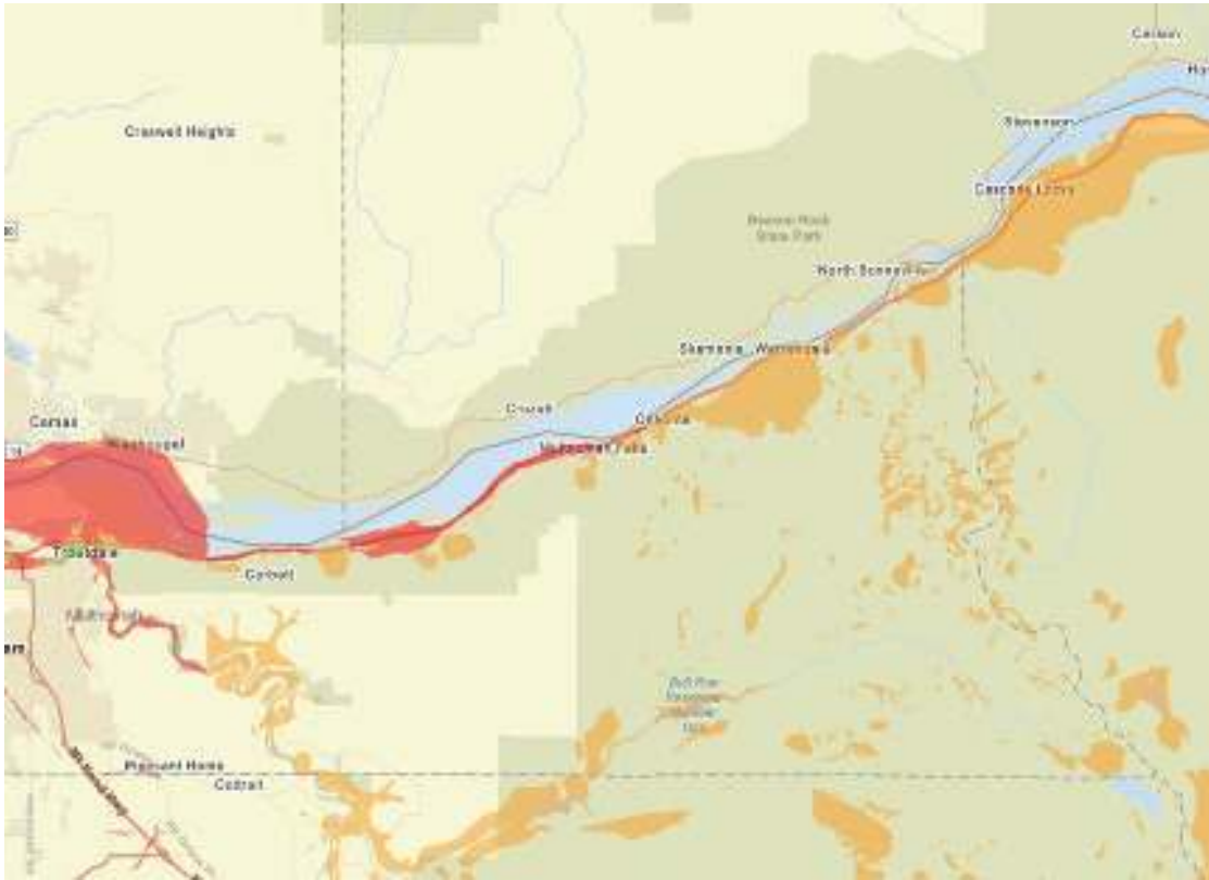
Figure 163 - Map showing soil liquefaction risk in the Eastern portion of Multnomah County. Red is the highest risk area, orange is moderate, and green has a lower risk. Map from DOGAMI's HazVu site.
