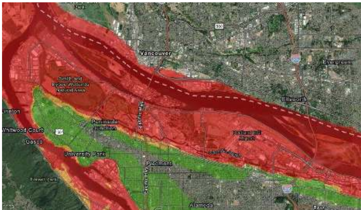
Figure 196 - Map showing soil liquefaction risk at the Port of Portland's critical community assets. Areas in red, which include the Portland International Airport and Terminal 6, have high risk of soil liquefaction. Map from DOGAMI HazVu site.
