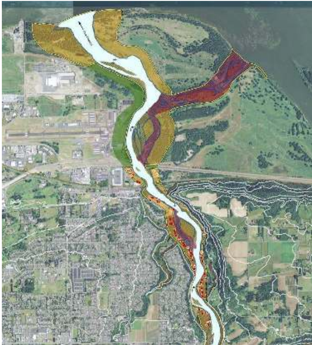
Figure 142 -- Map showing channel migration potential on the lower portion of the Sandy River in Troutdale. The yellow areas have risk from bank erosion in the next 100 years, the red areas have risk from the formation of a new river channel, the blue shaded areas are previous locations of the river channel at some point between 1955-2019, and the green areas are where built structures have eliminated risk of channel migration. The small red squares are the location of structures with some risk from the hazard. Map from DOGAMI report O-13-10 .
