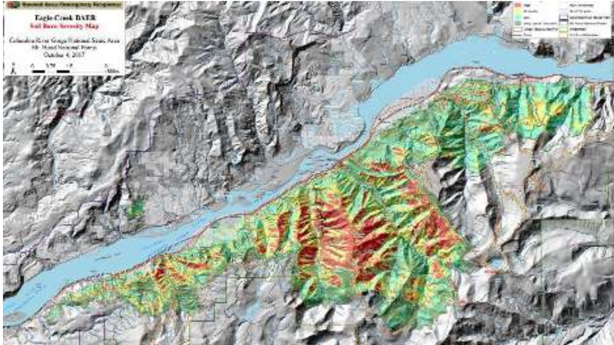
Figure 95 - Soil burn severity map from the 2017 Eagle Creek Fire showing locations with high severity in red, moderate severity in yellow, low severity in light green and very low to no impact in dark green. In low severity areas, ground cover is reduced but intact and the soil structure is unchanged, showing the normal mosaic of impacts in a large wildfire. Map from US Forest Service Eagle Creek Fire Story and Data page.
