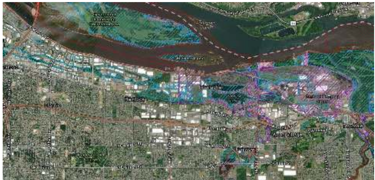
Figure 187 - FEMA National Flood Insurance Rate Maps in eastern districts showing 1% annual chance flood probability (100-year) in blue and the .2% annual chance flood area (500-year) in purple. The floodway is shown in red. Map from DOGAMI's HazVu site.
