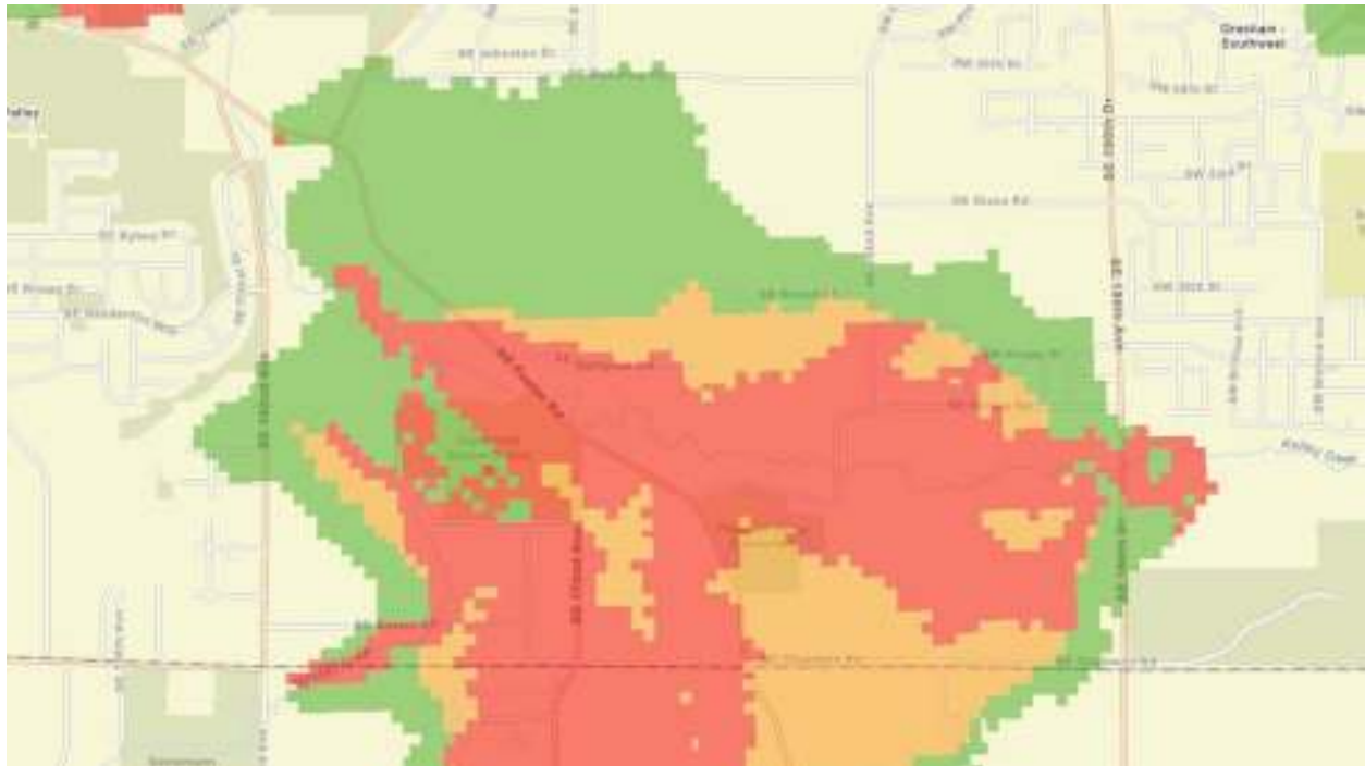
Figure 166 - Map showing soil liquefaction potential in the Pleasant Valley neighborhood. Red areas have the highest soil liquefaction potential, orange areas have moderate risk, and green areas have lower risk. Map from DOGAMI HazVu site.
