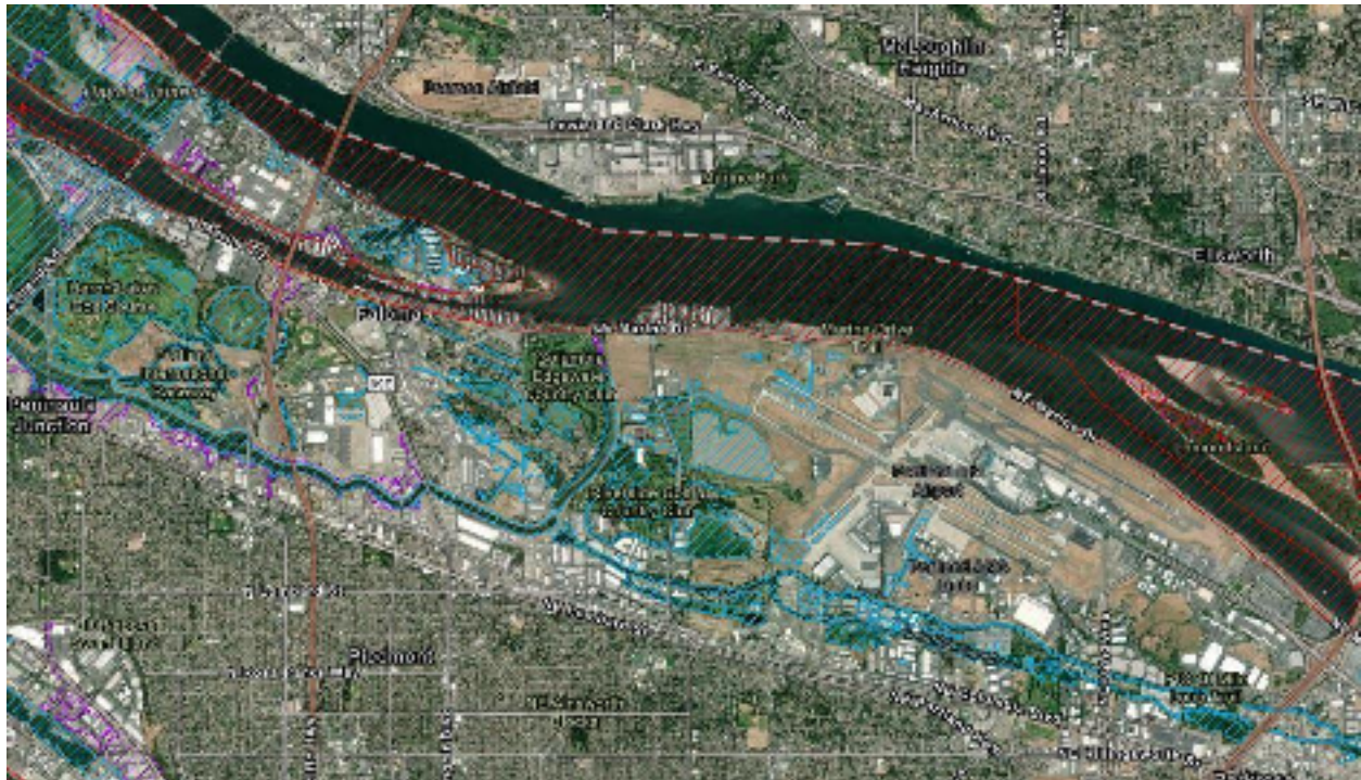
Figure 186 - FEMA National Flood Insurance Rate Maps in western districts showing 1% annual chance flood probability (100-year) in blue and the .2% annual chance flood area (500-year) in purple. The floodway is shown in red. Map from DOGAMI HazVu Site.
