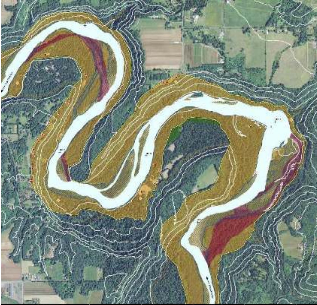
Figure 53 - DOGAMI map showing channel migration threat in the upstream portion of the Sandy River in Multnomah County. Yellow areas are at risk from erosion, red areas are areas at risk of new river channels forming, blue hatched areas are former channels, and green areas are areas that were once channels but have become disconnected from the channel movement process. The small red squares are locations of structures.
