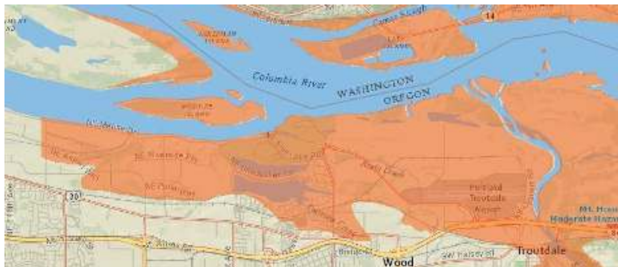
Figure 191 - Map showing risk from a volcanic lahar in an extra-large eruption (10,000-100,000 year event) of Mount Hood. Map from DOGAMI HazVu site. The study used for this image was limited to a fixed geographical boundary – effects from such a major lahar would extend further downriver beyond the western boundary indicated by the DOGAMI map.
