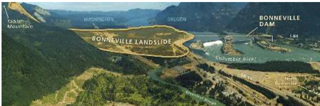
Figure 72 - Columbia River Gorge photo overlaid with an outline of the Bonneville Landslide. Image by Dan Coe, Washington Geological Survey/Washington Department of Natural Resources.
