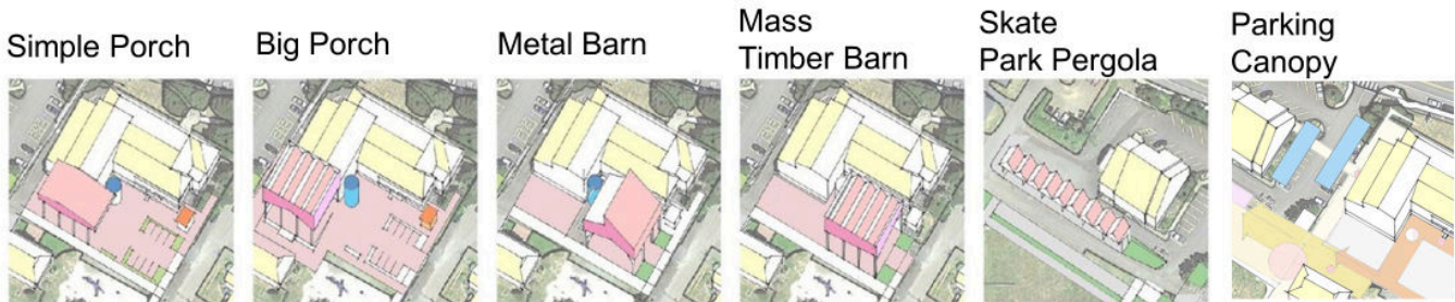
Figure 43. Six candidate options were considered to boost collection capacity to generate as much power as would be required to sustain the Southedge activities for up to 3 months when power generation is at its lowest.
