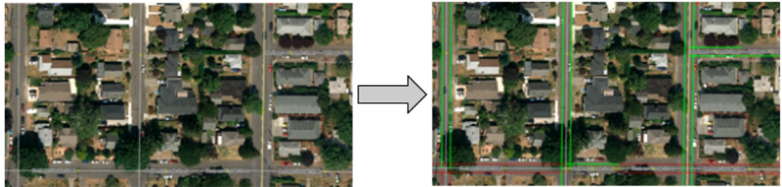
Figure 5-1 OSM data over aerial imagery in JOSM - sidewalks style activated to visualize sidewalk tags (right)
