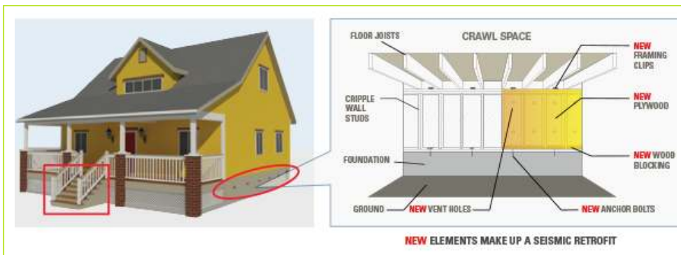
Seismic retrofit diagram. Source: California Earthquake Authority
