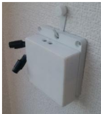
Floor, windows temp. sensor
